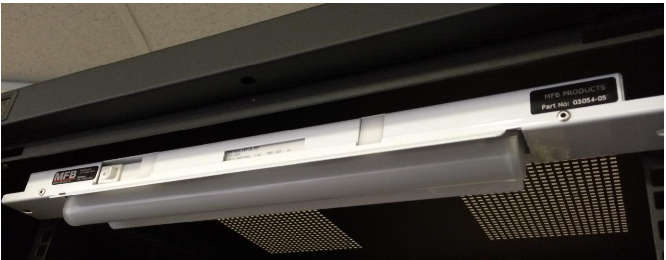
LED Light mounted in front 19" position
